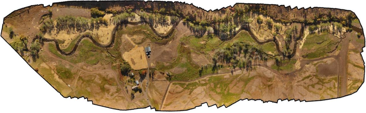
*CC 44 Southern Cross. Sponsor: CTUIR. Funders: BPA, CTUIR. Completed: 2016. Photos by Connor Stone (GRMW), Catherine Creek Subbasin. Photos demonstrate the new sinuous and complex channel that replaced the previously channelized section of Catherine Creek as well as the difference in technology gathering strategies to produce high resolution orthomosaics.*
