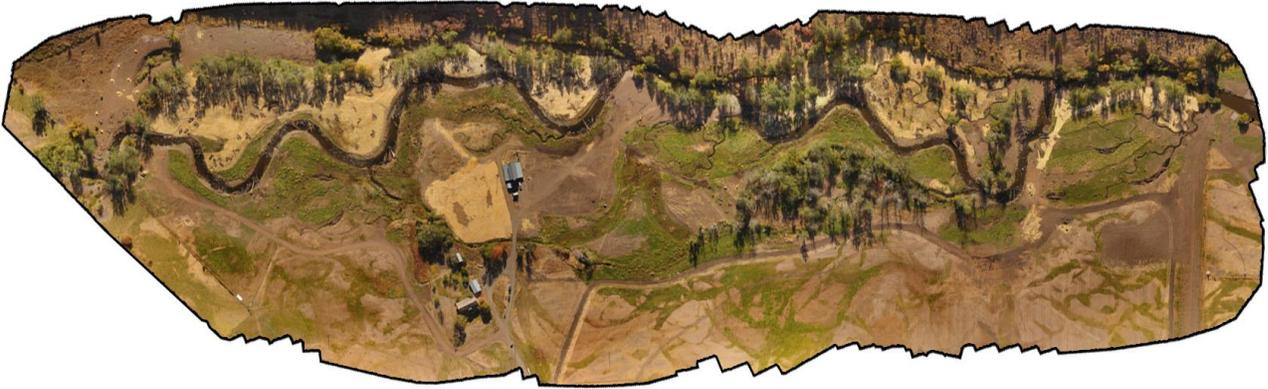
*CC 44 Southern Cross. Sponsor: CTUIR. Funders: BPA, CTUIR. Completed: 2016. Photos by Connar Stone (GRMW), Catherine Creek Subbasin. Photos demonstrate the new sinuous and complex channel that replaced the previously channelized section of Catherine Creek as well as the difference in technology gathering strategies to produce high resolution orthomosaics.*
