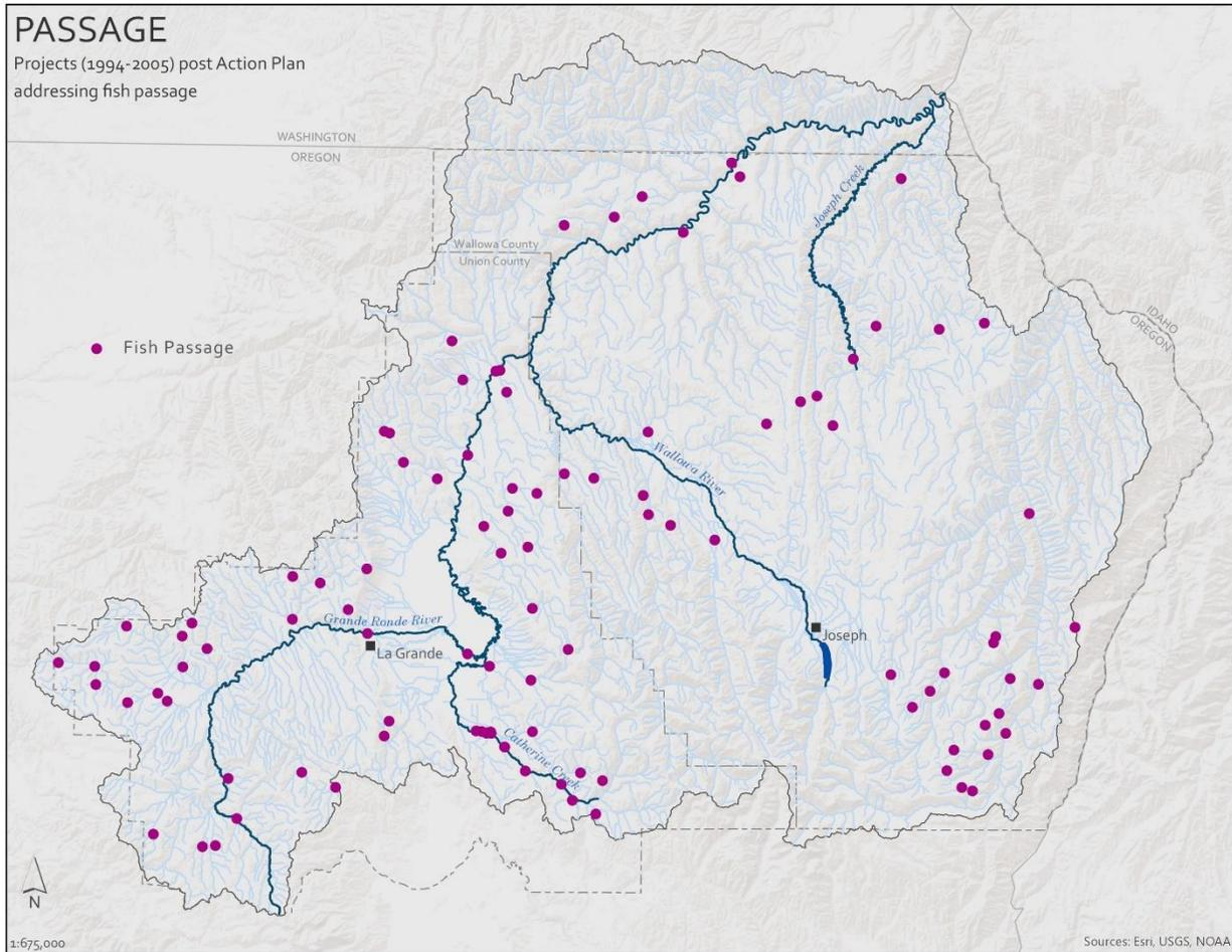
Seventy projects addressed fish passage. The majority of passage projects focused on improving road crossings, including road obliterations and relocations. Four fish ladders were constructed, and twelve projects addressed stream diversions. These projects were located throughout the subbasin, primarily on tributary streams; however, in the Catherine Creek Basin, the bulk of the projects were located on the mainstem.
